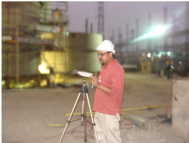
Photograph- 3: Noise Level Monitoring at Southern Side of Siddhirganj 335 MW Combined Cycle Power Plant Project
